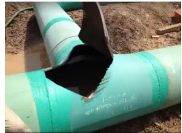
Hydrostatic Test Failure
