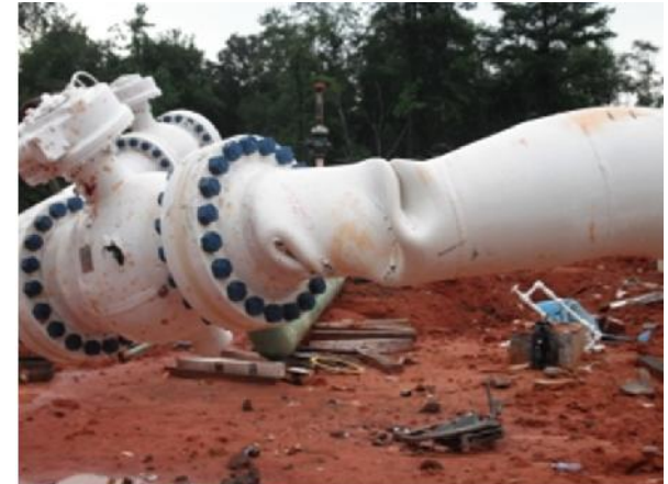
Pneumatic Test Failure
